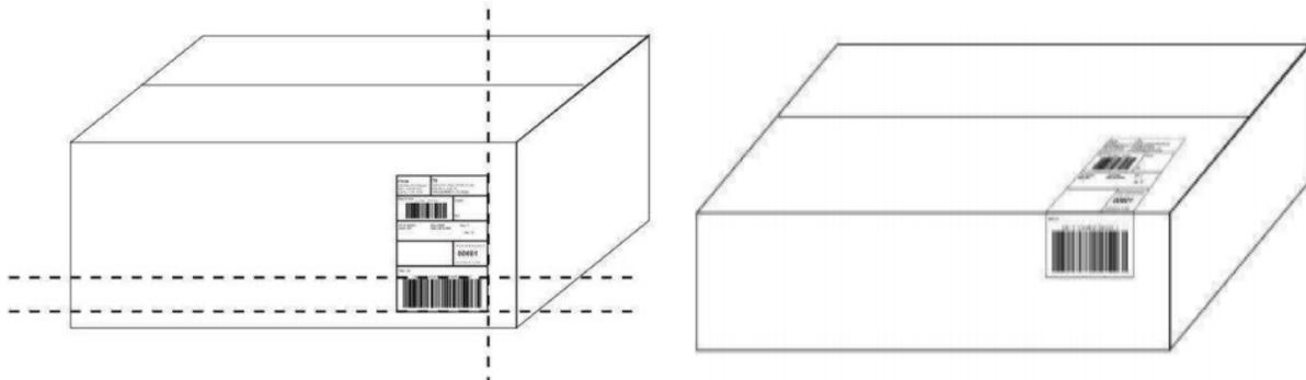
When consolidating, place the master GSI-128 label or a label indicating Master Pack onto the over-pack carton. Ensure each inside carton labeled individually with GS1-128 labels.
